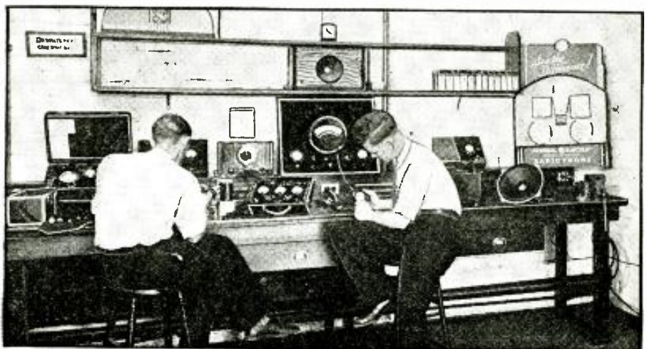
Fig. A. The work bench of the service shop of Brown and Nixon, Toronto, where the slogan is, "Honest Work at Fair Prices." Both partners have long experience in the game. They have built a good deal of the test equipment themselves, including an oscillator, megger, etc.
